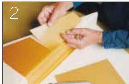
2 Positioning wax sheets onto model or tool. Use butt joints or the overlay and cut jointing technique.
