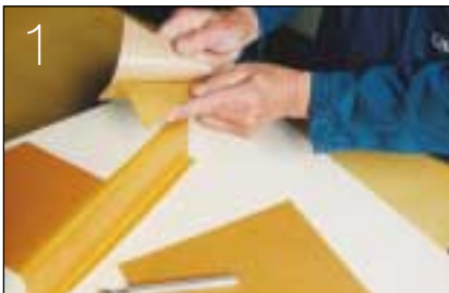
1 Removing the backing paper from the self-adhesive wax sheet.
