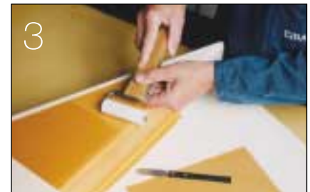
3 Rolling to extrude air bubbles.
