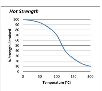
UV685 can withstand higher temperatures for brief periods (such as for paint baking and wave soldering processes) providing the joint is not unduly stressed. The minimum temperature the cured adhesive can be exposed to is -55°C (-67°F) depending on the materials being bonded.
